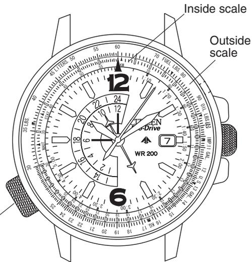
Crown for turning the outer scale
