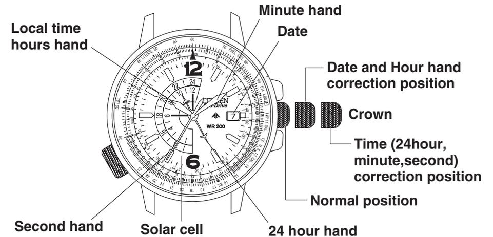
\*If the crown is of the screw-type, set the time and calendar after first loosening the screw. Retighten the screw after the time and calendar have been set.
